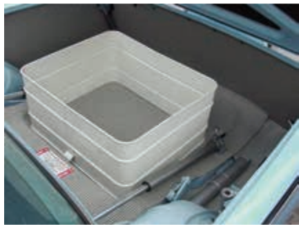
Photo showing Trunk Boards and Burtex floor covering with tub in place.
